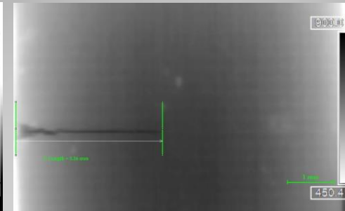
Surface crack length after 6549 cycles
