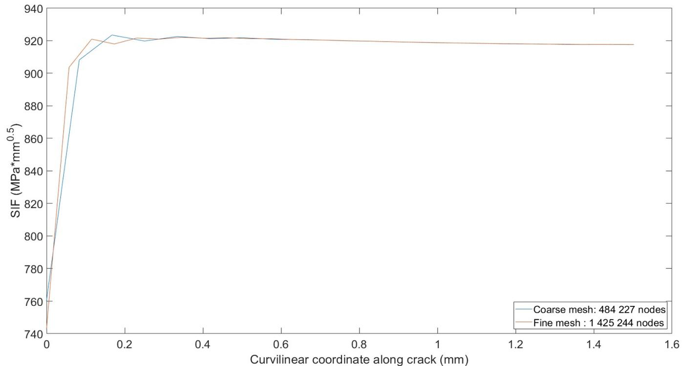
Figure 14 : SIF calculated for two degrees of mesh refinement
