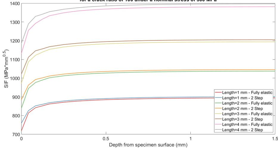
SIF calculated for four crack lengths and both material models for a crack ratio of 6 under a nominal stress of 300 MPa
