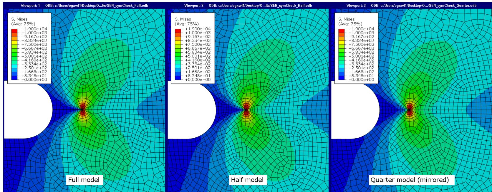
Figure 11 : Max. principal stress calculated for the three models
