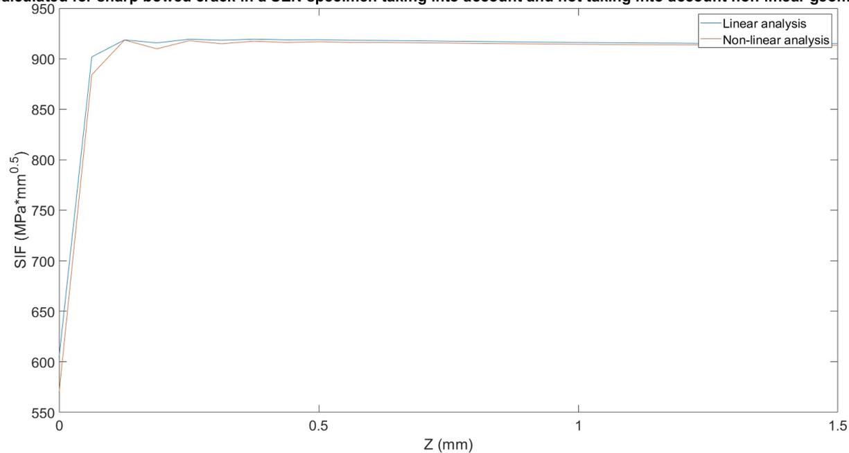
Figure 12 : SIF calculated with and without considering geometric non-linearity
