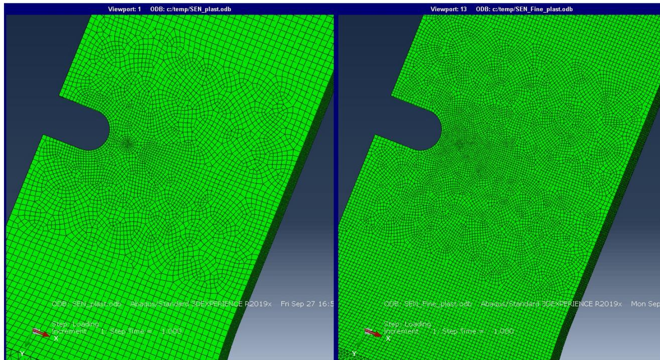
Figure 13 : A coarse and a fine mesh
