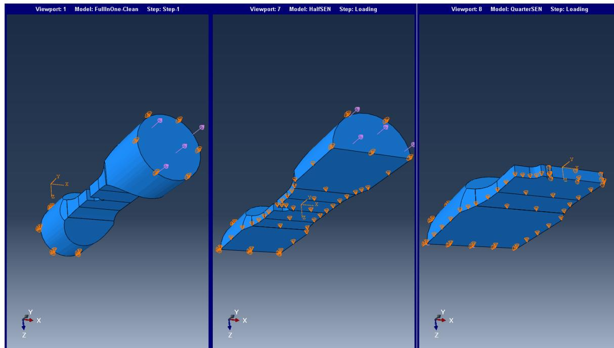
Figure 9 : Three models exploiting various symmetry planes
