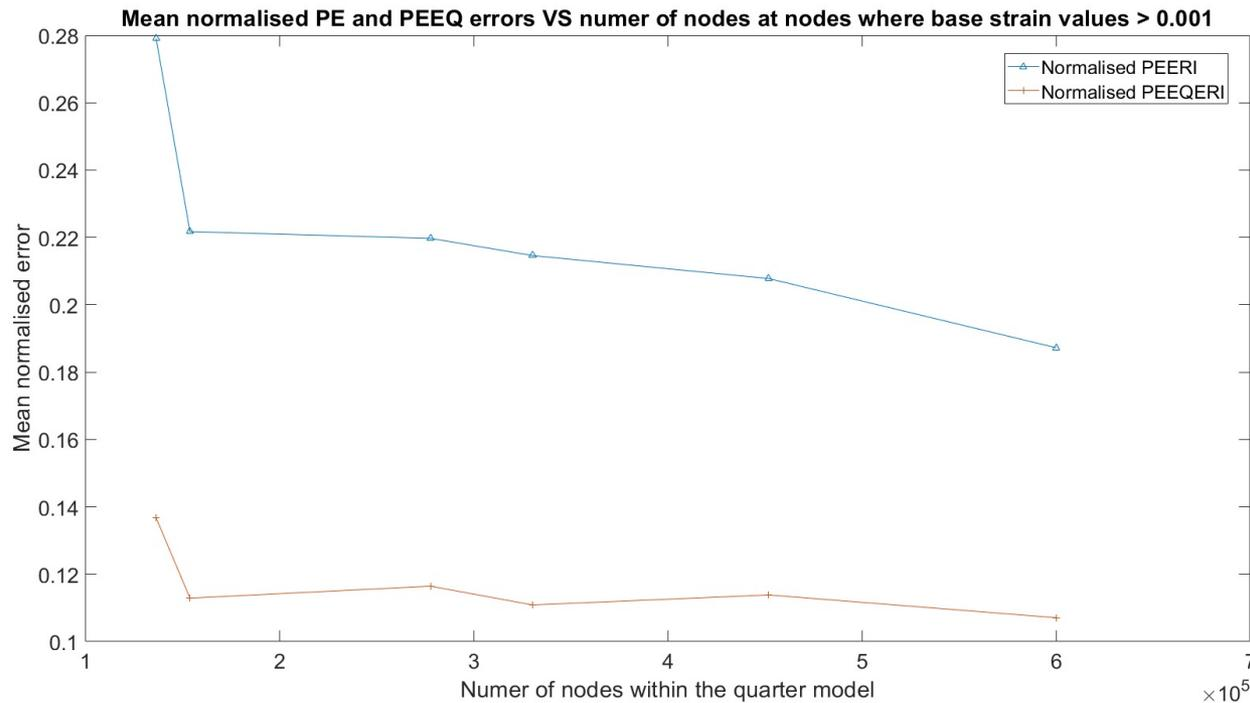
Figure 16 : Mean normalised plastic strain errors according to Abaqus
