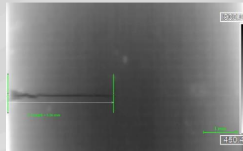
Image of surface crack length after 6549 cycles
